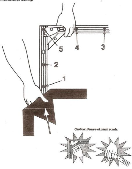
For removal of the screen, reverse the steps and take each snap pin off individually. Be careful when removing snaps to not rip the fabric.
